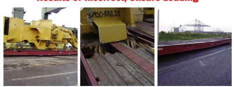
There must be a load on the gooseneck to prevent the roll trailer from tipping backwards. This is generally caused by too much load past the wheel cluster.
